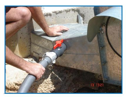
**F.** Connect the suction hose between the pipe connected to the silo headspace (downcomer) to the inlet point at the bottom of the fumigation box. Ensure that the valve is fully open .
