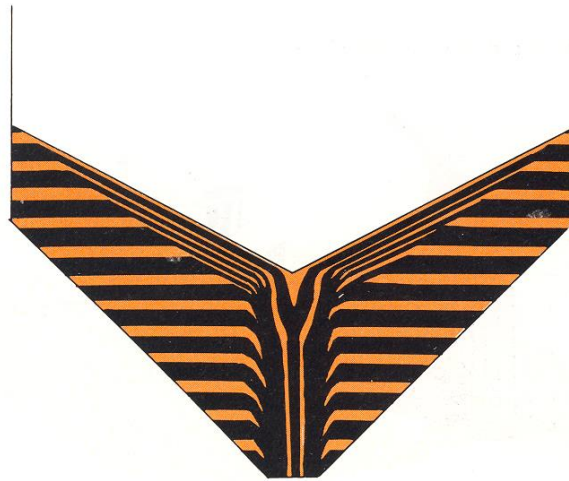
“FUNNEL FLOW” of Grain out of a typical silo.
